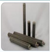
Pleated SS 316/304 mesh cartridges offer the convenience of having a larger filtration area within a small enclosure since the media is pleated and enclosed within a cage of suitable diameter. These cartridges are absolutely non-particle shedding & hence prevent any product contamination. They are suited for filtration of viscous fluids at high temperatures & high pressures
