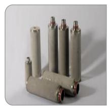
Sintered SS 316 cartridges. Made from compacted pre-graded SS 316 / SS316L granules. Welded end caps provided to prevent filtrate bypass. Absolutely non-particle shedding & hence prevent any product contamination. They are ideally suited for high temperature & high pressure applications. They can be cleaned by simple back-flushing with water or suitable medium, thereby providing trouble free operation for a number of years.
